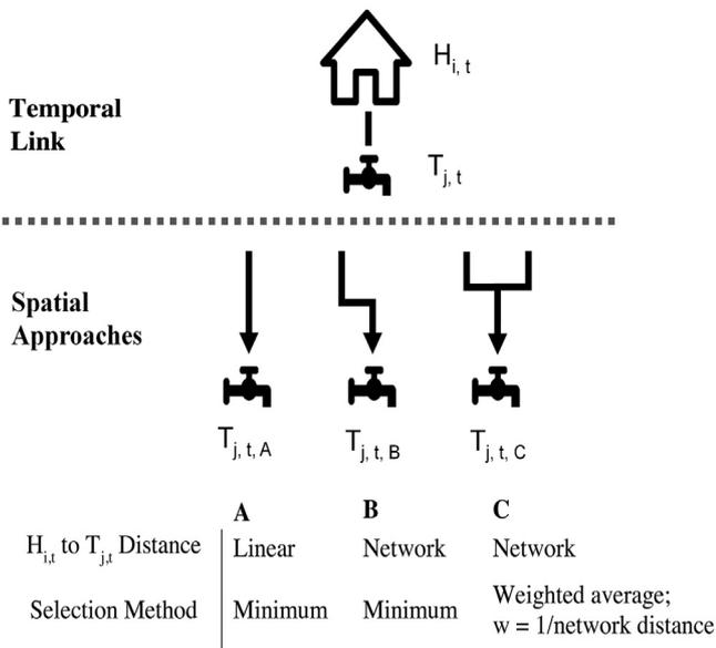
**Fig. 1.** Schematic of three spatial approaches (A, B, and C). Households ( $H_i$ ) and potential source taps ( $T_j$ ) are first selected based on same-day sampling ( $t$ ), and then source taps are selected based on measures of proximity (Euclidean and network distances).
